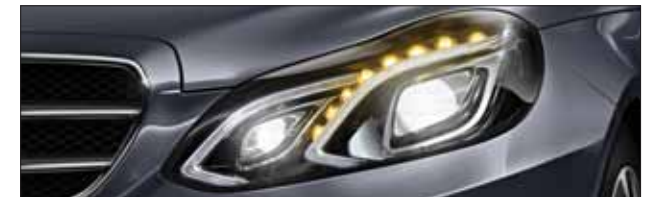
Driving lights and turn indicators switched on, daytime running lamps dimmed, LED Intelligent Light System
