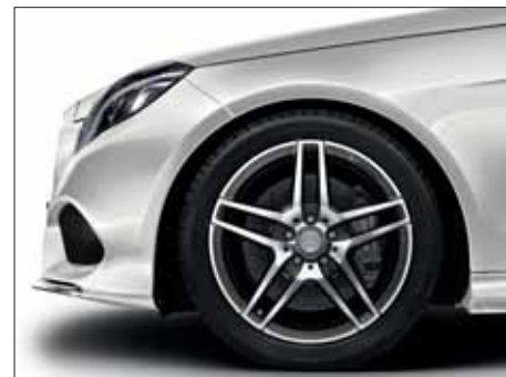
AMG 5-twin-spoke wheel, High Sheen Aluminum, Silver Wheel: 8.5 J x 18 ET 48 | Tyre: 245/40 R18 XL
