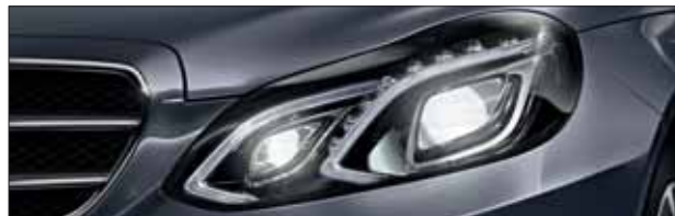
Driving lights switched on and daytime running lamps dimmed, LED Intelligent Light System
