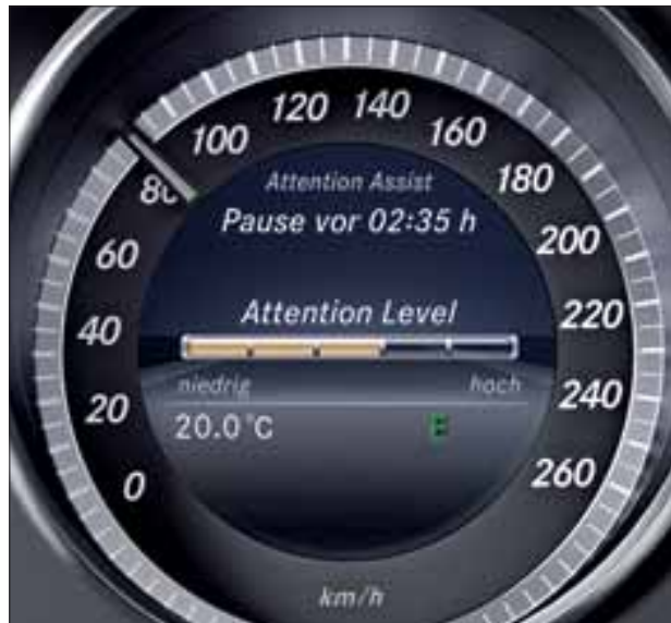
If signs of increased driver inattention or drowsiness are detected, ATTENTION ASSIST advises taking a break
